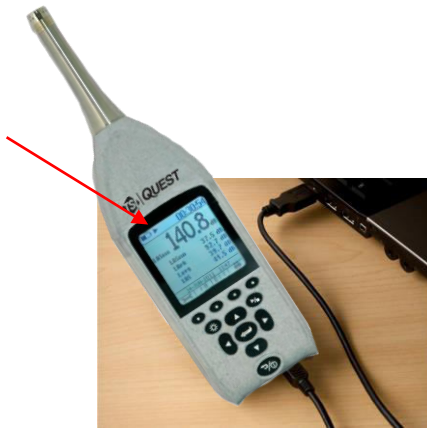
Figure 2-3: Charging state for SE-400 Series
