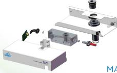
Optical CPM module for evaluation in real time of several particulate size fraction
