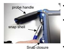
Fig. 26: Wohler A 550 INDUSTRIAL with open probe compartment
