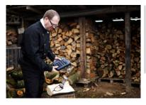
Fig. 45: Wood moisture measurement with Probe Wohler HBF 420.
