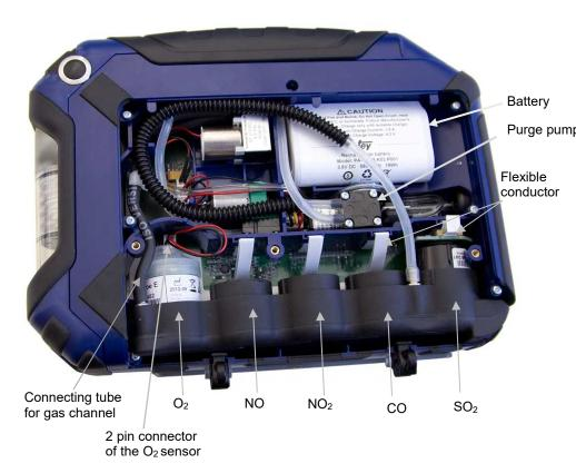
Fig. 72: Bottom of the analyzer without cover
