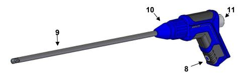
Fig. 4: Probe handle with gas probe 295 mm
