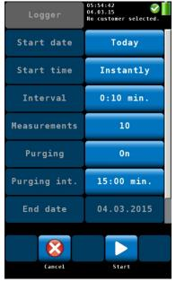
Fig. 58: Configuration of the logger measurement
