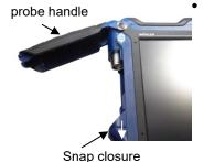
To open the probe compartment pull down the snap closure under the black probe handle.
