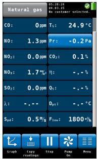
Fig. 39: Values screen with speed and flow
