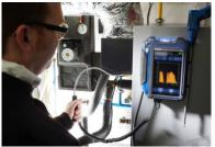
Fig. 50: Spillage test: Searching for condensate
