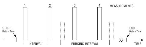
Fig. 57: schematic representation of a logger measurement
