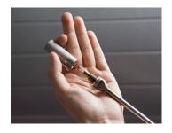
The gas probe 1,000 mm has an in-stack sinterfilter for dust protection. It removes dust (> 20 ym) from the sample gas to protect the analyzer against heavy dust loads.
