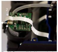
Fig. 73: Sensor with locking mechanism (1) and flexible conductor (2)
