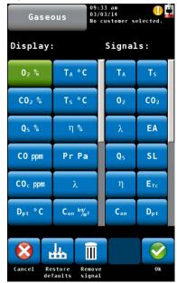
Fig. 61: Configuration of the readings segment.
